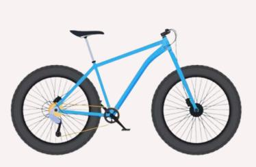
Fat bikes are bicycles with oversized tires, typically 3.8 inches or wider, that allow for better traction on soft, unstable terrain such as sand or snow. They have wider rims, frames, and forks to accommodate the larger tires, and are often used for adventure and endurance cycling.
